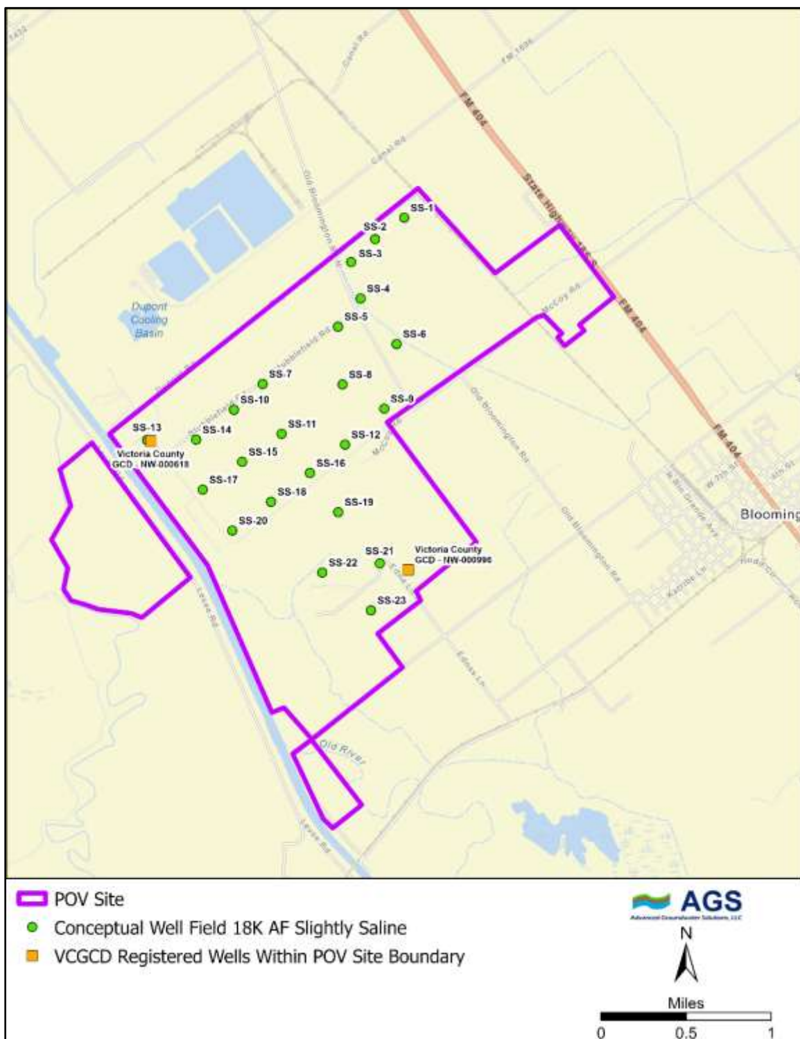
Figure 2. POV slightly saline conceptual wellfield and VCGCD-registered wells within the POV site.
